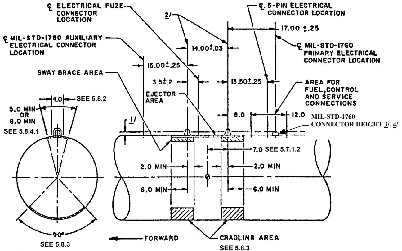
1/ A minimum 0.625-inch clearance shall be provided between the rack lower surface and the store upper surface. This clearance shall not apply to rack hooks, braces, ejectors, store lugs, or service connections.
