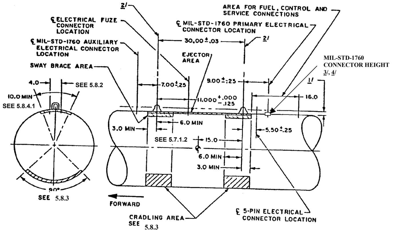
1/ A minimum 0.625-inch clearance shall be provided between the rack lower surface and the store upper surface. This clearance shall not apply to rack hooks, braces, ejectors, store lugs, or umbilical connections.
