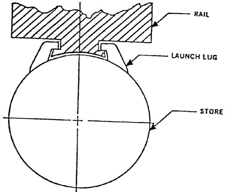
FIGURE 12. Example of external U-shaped shoe.
