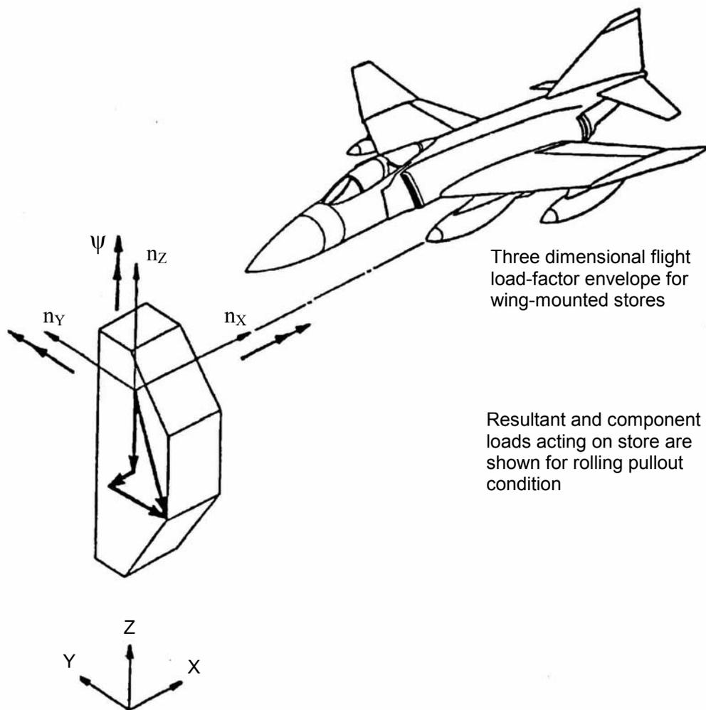
NOTE: Loads, load factors, and dimensions are positive when acting aft, to the right (looking forward) and up. Angles, moments, angular accelerations and angular velocities about axes parallel to the reference axes follow the right-hand rule.
