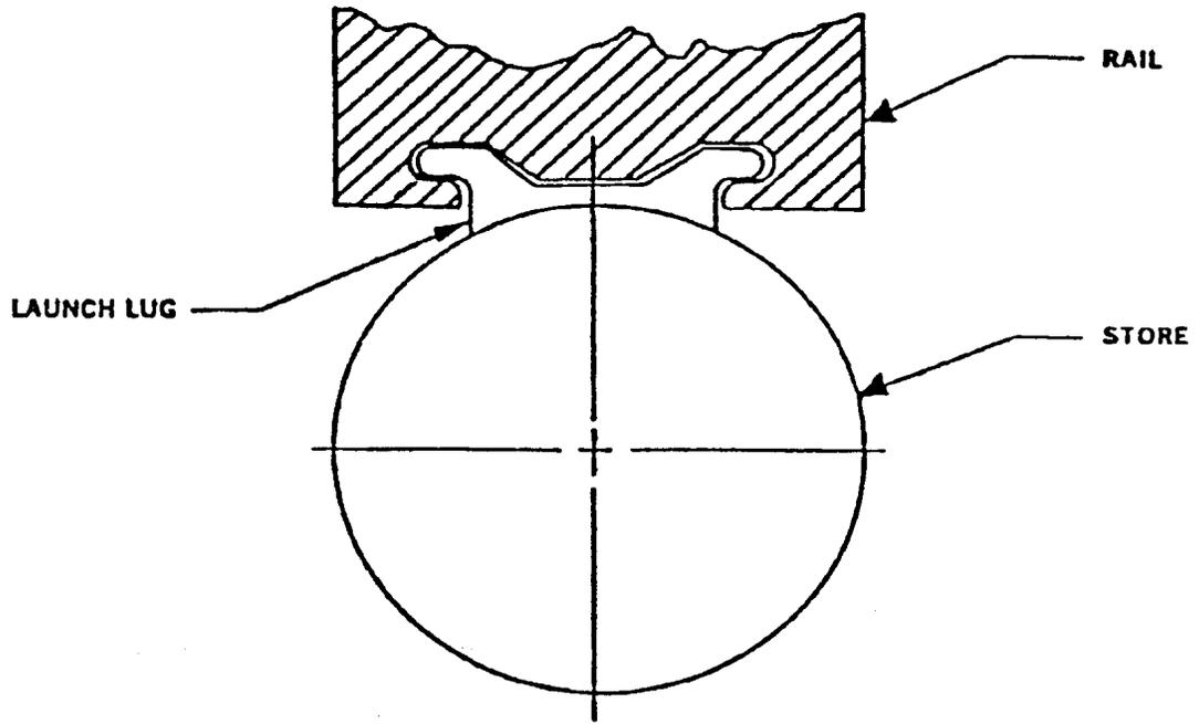
FIGURE 11. Example of internal T-shaped hangar.
