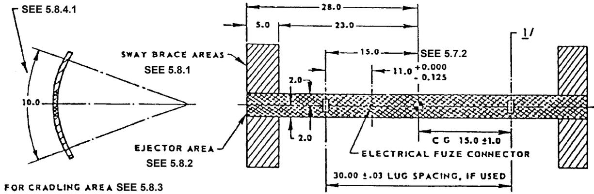
1/ If used, lug and lug well axes shall be normal to the store longitudinal axis within  $\pm 1/2^\circ$  and in the same plane within  $\pm 1/2^\circ$ .
