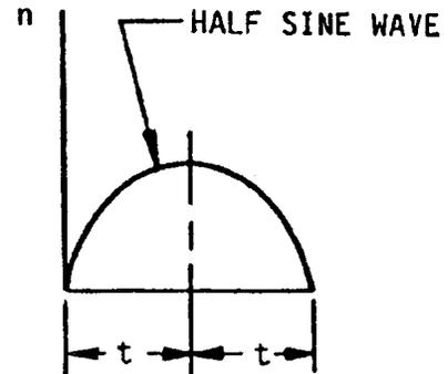
FIGURE 14. Time-load factor curve.
