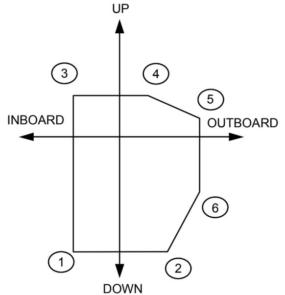
FIGURE B-1. Aircraft angles of attack and sideslip at specific load envelope points for wing or sponson-mounted stores.
