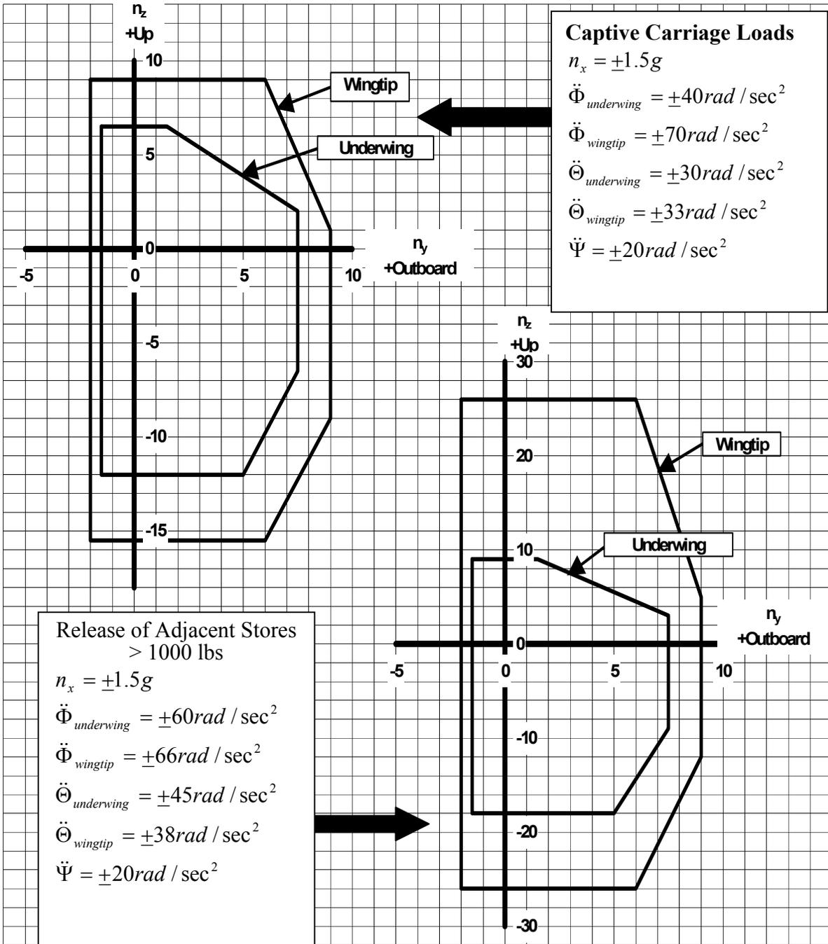
FIGURE A-3. Design flight inertia limit load factors for wing or sponson-mounted stores. Data applies at the store center of gravity (cg).
