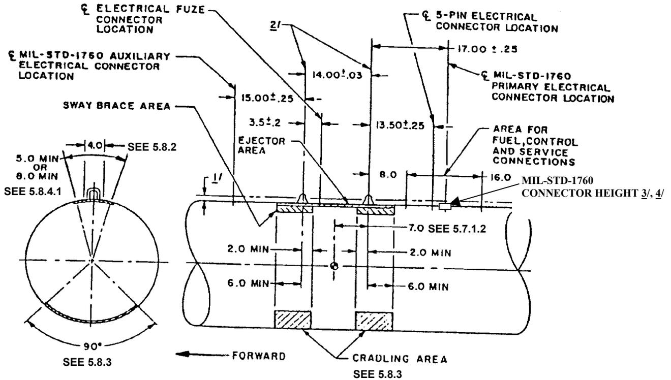
1/ A minimum 0.625-inch clearance shall be provided between the rack lower surface and the store upper surface. This clearance shall not apply to rack hooks, braces, ejectors, store lugs, or service connections.
